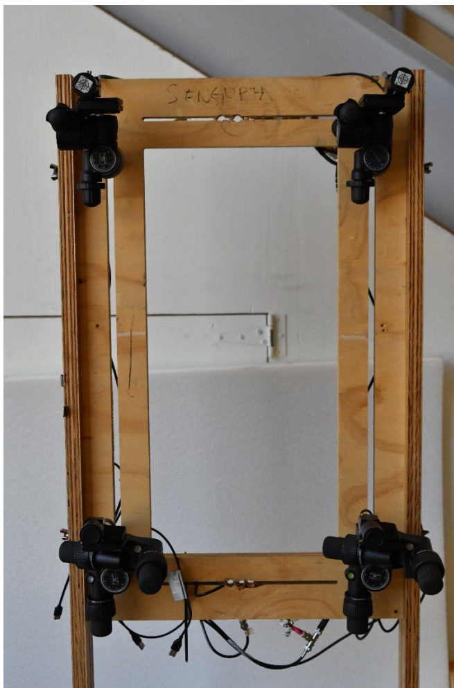
Fig. 5 Quadrocular EBC stereo setup: four SilkyEvCam cameras are mounted on a custom stand. Counterclockwise starting from the top right, serial nos. for each part are: 291, 290, 289, and 288.
